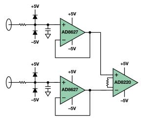
Figure 2. The AD8627 JFET operational amplifier used as a buffer for low input bias current.
