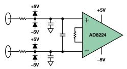
Figure 3. The AD8224 JFET instrumentation amplifier offers low input bias current.
