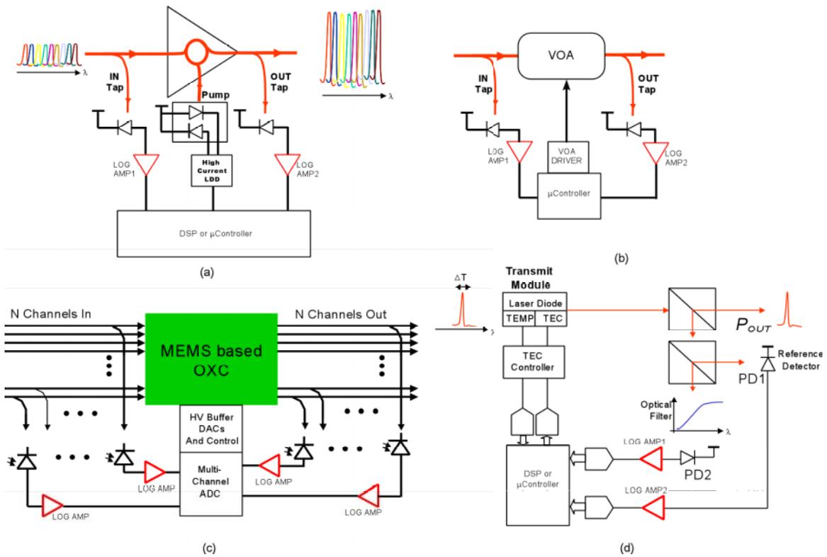
**Figure 4. Several Log Amp Optical Power Monitoring Applications. a) An Optical Amplifier Gain Measurement, b) VOA Attenuation Measurement, c) MEMS Optical Cross Connect Application, d) Tunable Laser Application.**
