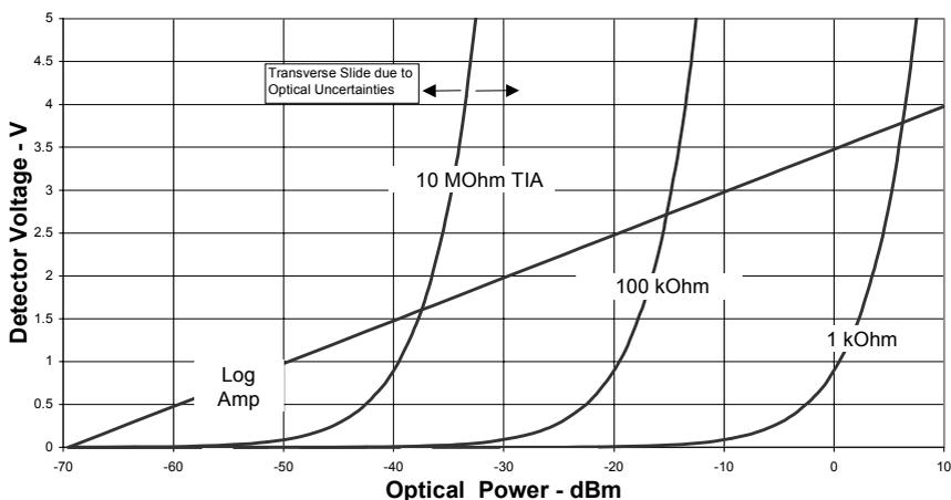
**Figure 2. Transfer Function of Transimpedance (TIA) Amplifier versus Log Amp. Coupling uncertainty, responsivity deviations and fiber loss can cause a transverse slide of the transfer function often requiring multi-point calibration.**
