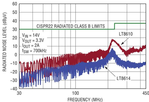
Figure 3. Comparison of radiated emissions for LT8614 and LT8610
