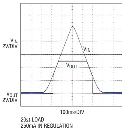
The LT8614's low minimum on-time of 30ns enables large step-down ratios even at high switching frequencies. As a result, it can supply logic core voltages with a single step-down from inputs up to 42V.
