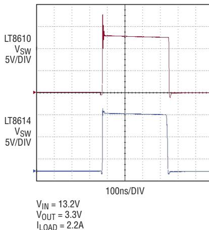
Figure 6. Dropout behavior of switch node for LT8614 and LT8610
