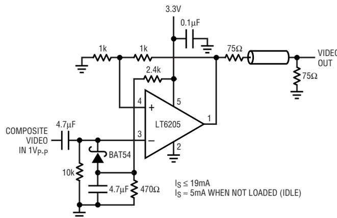
Figure 4. AC-coupled clamped-video amplifier powered from 3.3V
