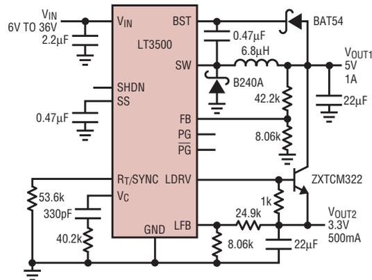
**Figure 1. Dual step-down converter for 5V at 1A and 3.3V at 1A**
