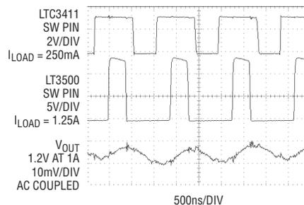
Figure 9. Synchronized switch waveforms for Figure 8 application
