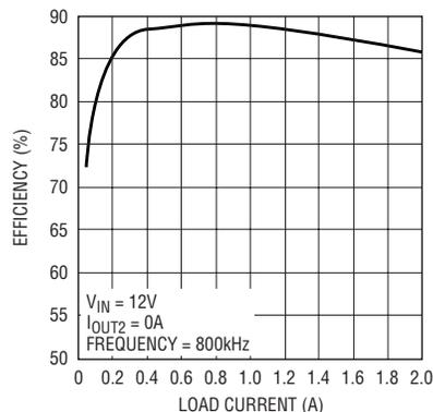
**Figure 2. LT3500 switching regulator efficiency**
