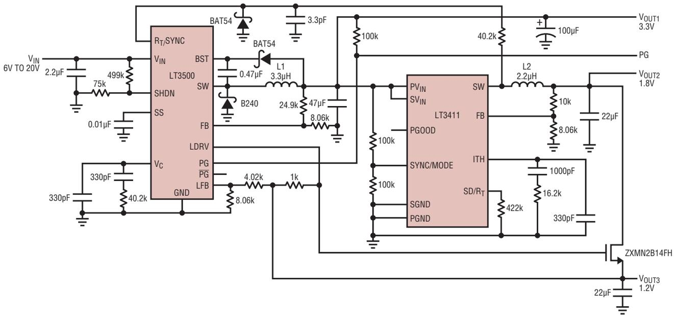
Figure 8. Triple output application
