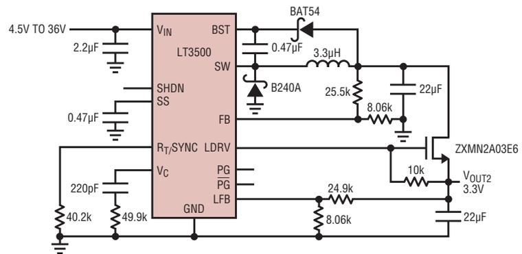
**Figure 6. High efficiency linear regulator**
