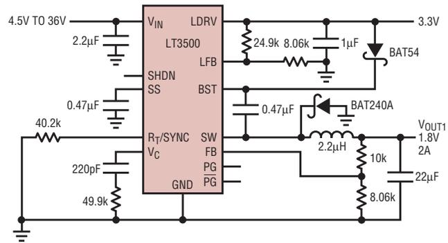
**Figure 5. 1.8V/2A step-down regulator**
