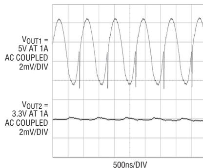
**Figure 3. 5V and 3.3V output ripple waveforms**
