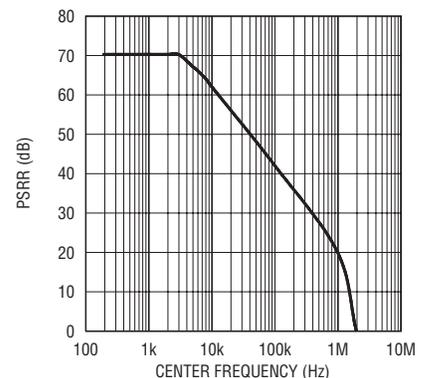
**Figure 4. PSRR vs Frequency for V<sub>OUT2</sub> for the application shown in Figure 1**
