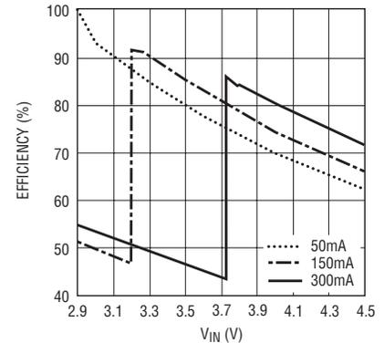
Figure 1. Efficiency vs  $V_{IN}$  for various LED currents
