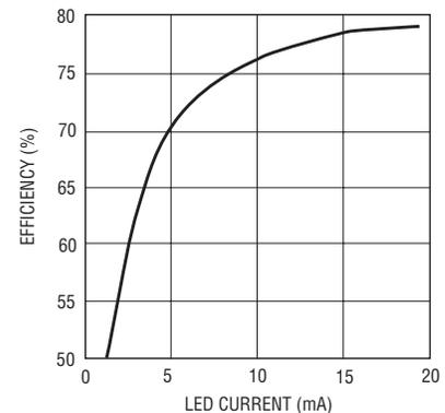
**Figure 10. Efficiency of the LED driver in Figure 9**
