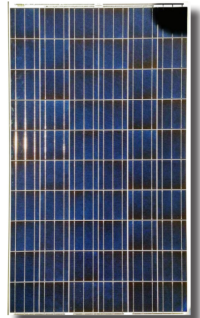
Figure 3. The solar panel shaded in top right corner
