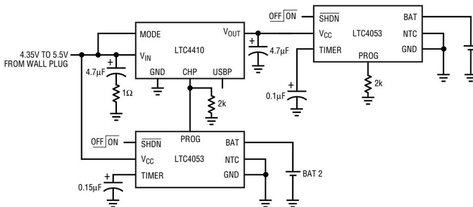
Figure 2. Priority dual battery charging with a wall adapter
