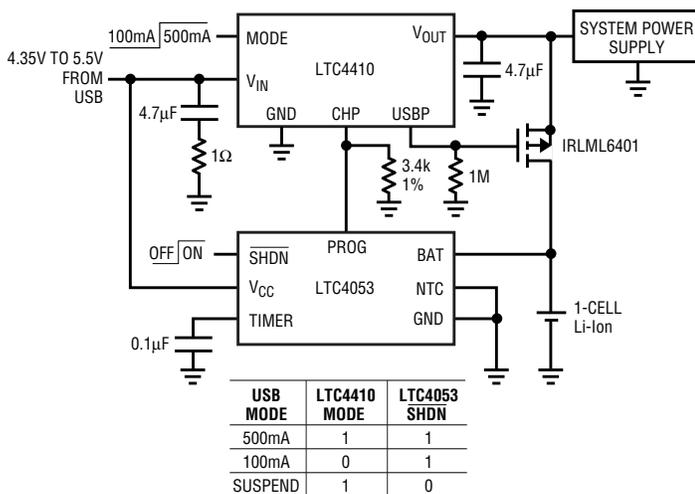
Figure 1. USB power manager and battery charger
