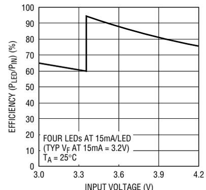
Figure 6. 4-LED main panel efficiency vs battery voltage
