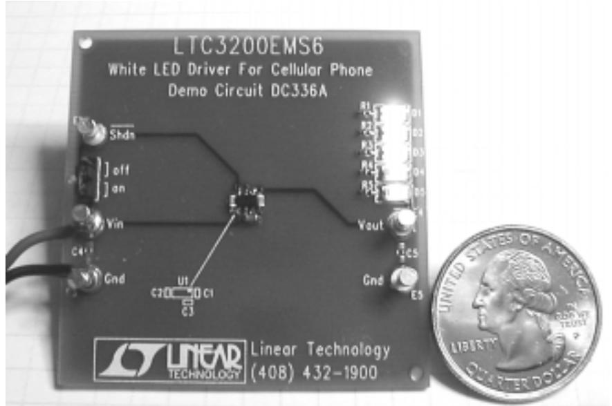
Figure 1. LTC3200 evaluation circuit
