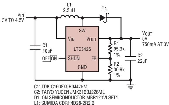
**Figure 4. Compact application circuit for V<sub>OUT</sub> at 5V**
