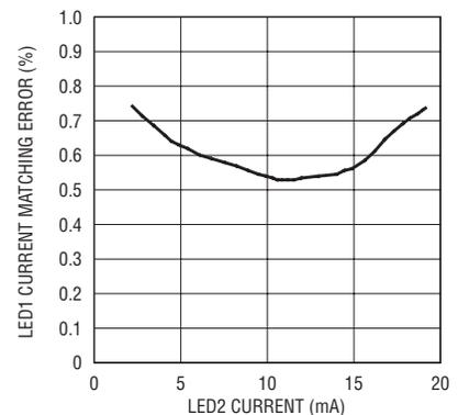
Figure 2. Typical current matching between LED1 and LED2
