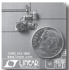
**Figure 5. Photograph of demo board of circuit in Figure 4—board area is 10mm × 12mm**
