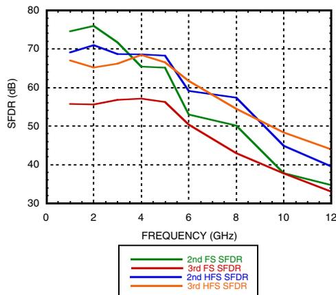
**Hold-Mode THD vs. Frequency & Input Power @  $f_{clk} = 1 \text{ GHz} @ +6 \text{ dBm}$**
