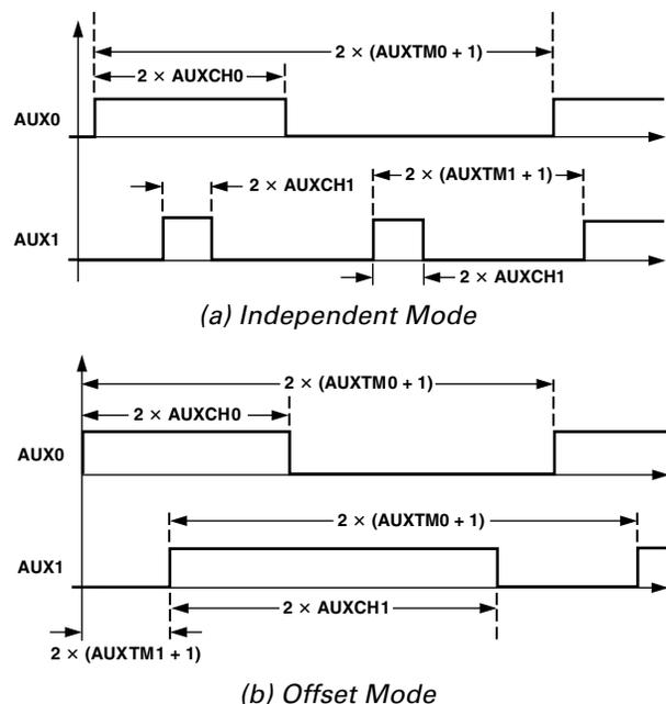
Figure 16. Typical Auxiliary PWM Signals.
