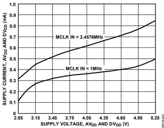
Figure 7. I<sub>DD</sub> vs. Supply Voltage
