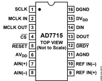
Figure 3. Pin Configuration
