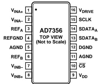
Figure 2. Pin Configuration
