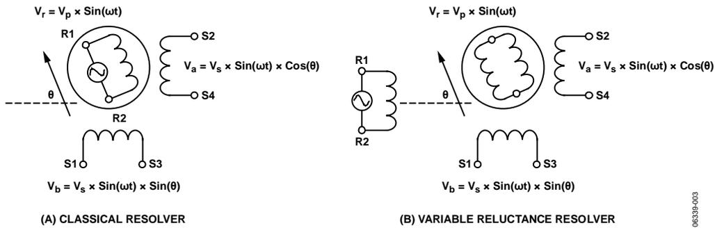
Figure 3. Classical Resolver vs. Variable Reluctance Resolver
