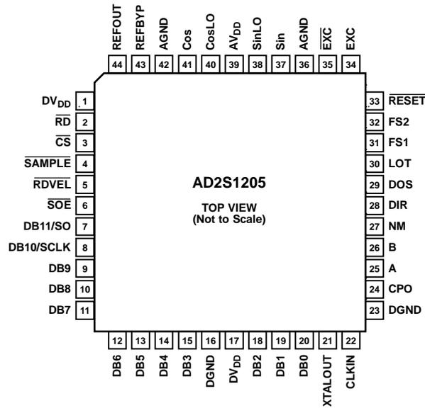
Figure 2. Pin Configuration
