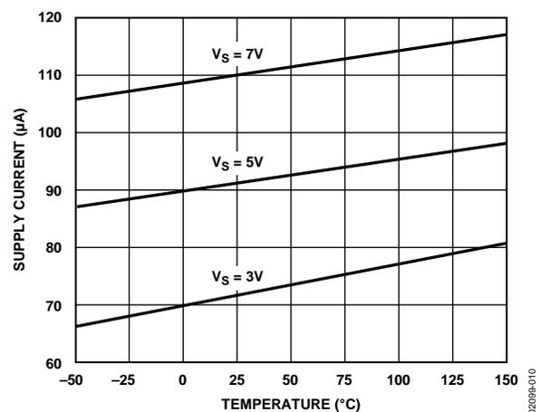
Figure 9. Supply Current vs. Temperature,  $V_{OUT}$  = Low
