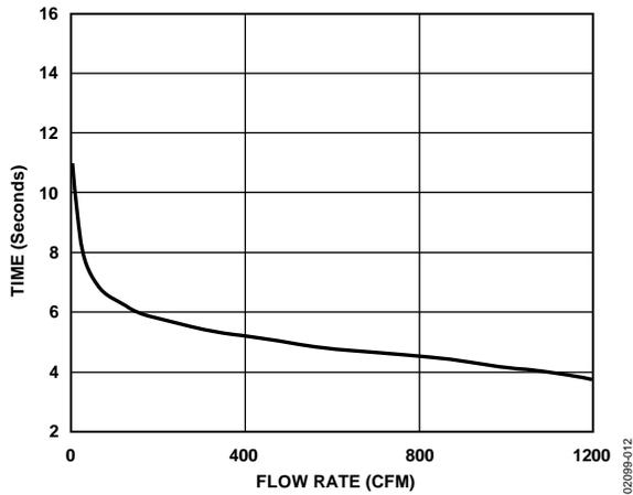
Figure 11. Time vs. Flow Rate, Thermal Response
