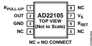
Figure 3. Pin Configuration
