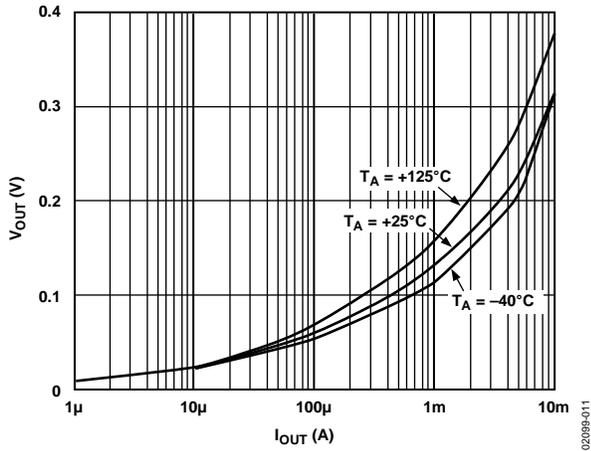
Figure 10.  $V_{out}$  vs. Output Current ( $I_{out}$ ),  $V_{out} = Low$
