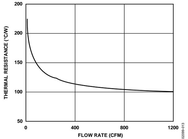
Figure 12. Thermal Resistance ( $\theta_{JA}$ ) vs. Flow Rate
