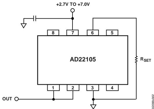
Figure 14. Typical Application Circuit
