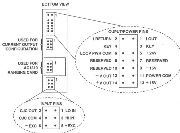
Figure 4 . Model 3B Series Module, with pin-out assignments.
