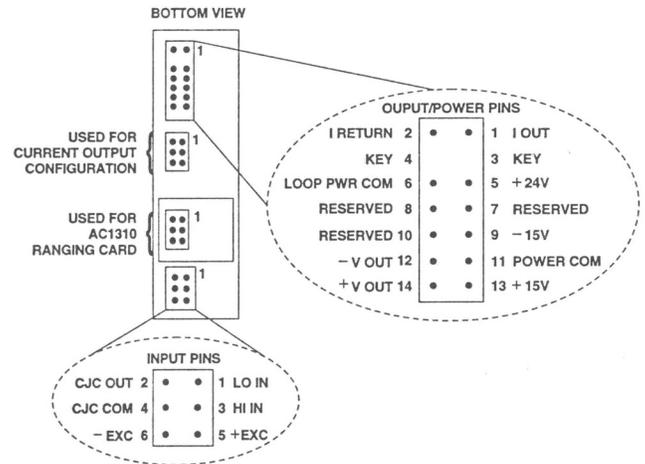
Figure 4 . Model 3B Series Module, with pin-out assignments.
