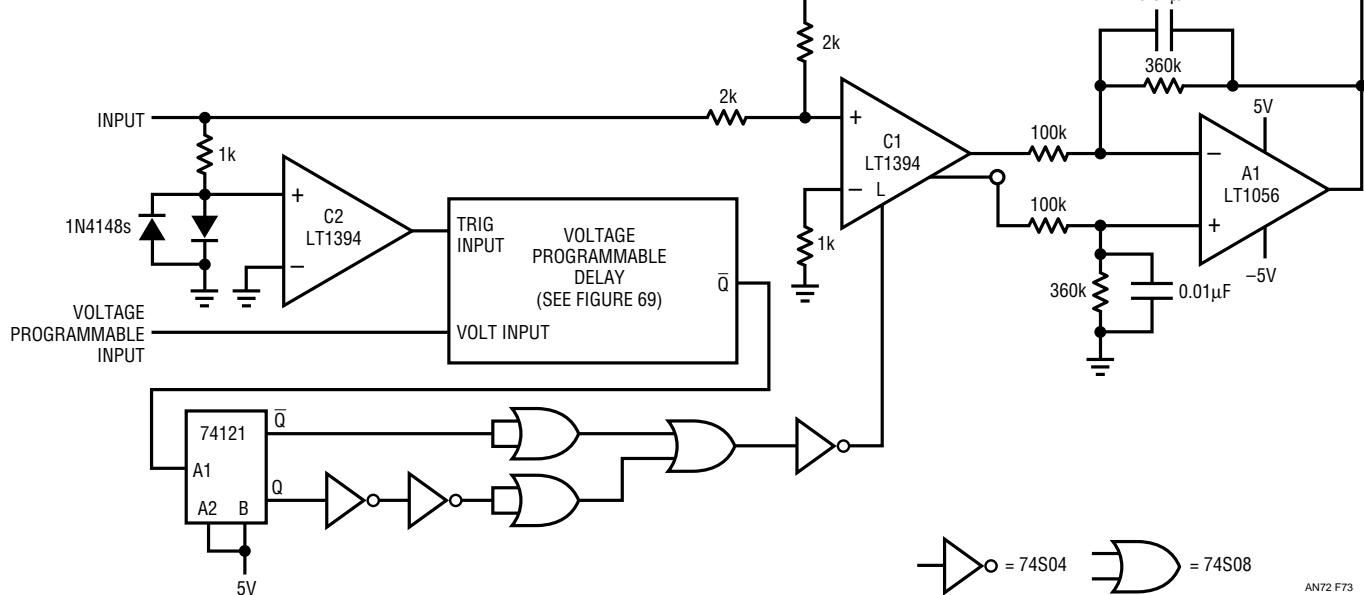
**Figure 73. 10ns Sample-and-Hold for Repetitive Signals. Feedback Loop Around Comparator and Programmable Delay Allow Controllable Sampling of Input**
