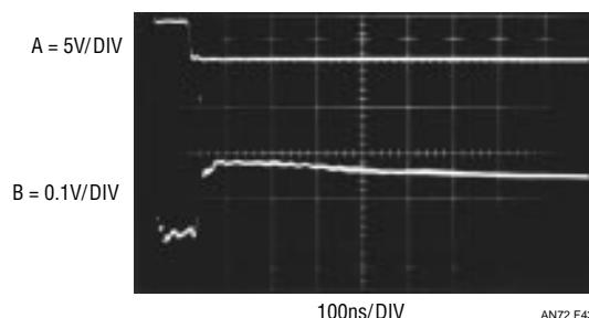
Figure 43. Response of  $10\mu F$  Aluminum Capacitor
