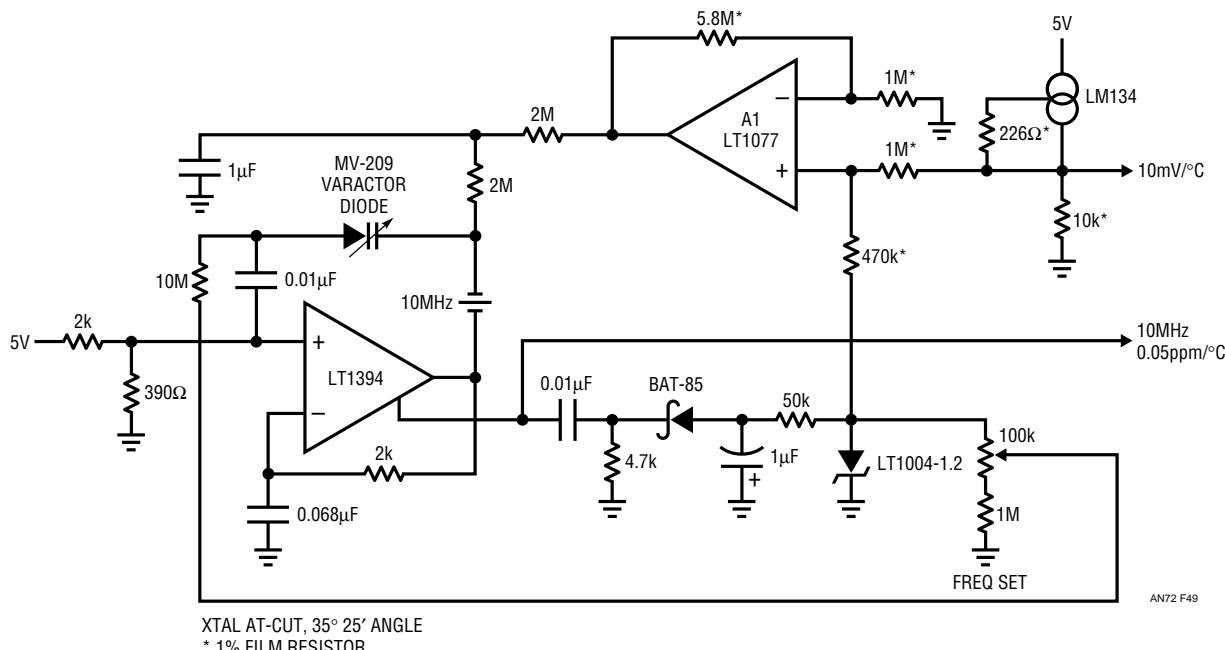
Figure 49. Temperature-Compensated 10MHz Crystal Oscillator.
