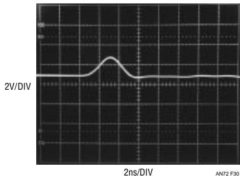
Figure 30. 150MHz Oscilloscope ( $t_{RISE} = 2.4\text{ns}$ ) with Direct Connection Responds to the Test Pulse
