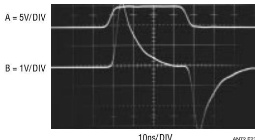
**Figure 23. Test Circuit Output with FET Probe**
