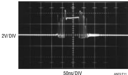
**Figure 11. 3pF Stray Capacitive Feedback with  $3\text{k}\Omega$  Source Can Cause Oscillation**
