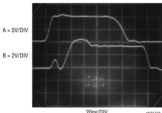
Figure 15. Input Common Mode Overdrive Generates Odd Outputs
