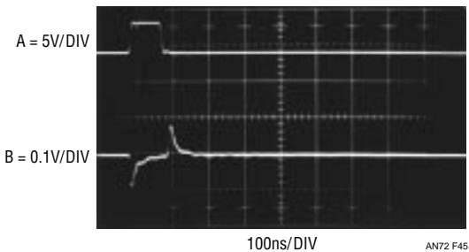
**Figure 45. Response of  $10\mu\text{F}$  Aluminum Paralleled by  $0.01\mu\text{F}$  Ceramic**
