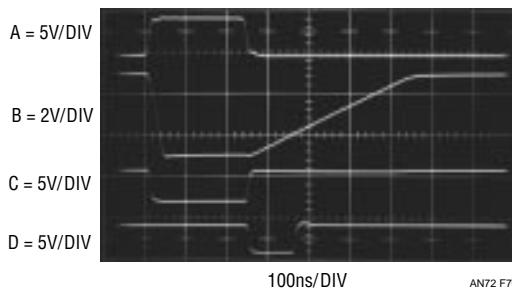
**Figure 70. Voltage-Controlled Delay's Waveforms. Programming Voltage Determines Delay Between Input (Trace A) Falling Edge and Output (Trace D) Rising Edge. High Linearity Timing Ramp (Trace B) Permits 1ns Accuracy and 100ps Repeatability**
