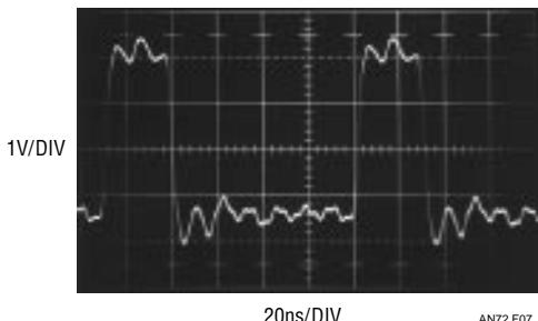
Figure 7. Typical Results Due to Poor Probe Grounding
