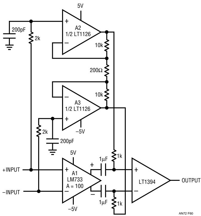
Figure 65. Parallel Preamplified Paths Allow 18ns Comparator Response to  $500\mu\text{V}$  Overdrive
