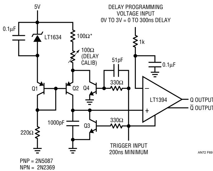
**Figure 69. Fast, Precise, Voltage-Controlled Delay. Emitter Switched Current Source Has Clean, Predictable Dynamics**
