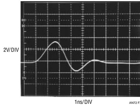
**Figure 28.** Test Pulse Measures Only 3V High on a 250MHz 'Scope with Significant Waveform Distortion. 290MHz 10 $\times$  Probe Used
