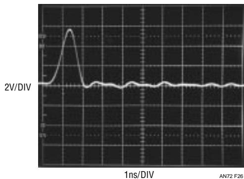
**Figure 26.** The Test Pulse Appears Smaller and Slower on a 350MHz Instrument ( $t_{RISE} = 1\text{ns}$ ). Deliberate Poor Grounding Creates Rippling After the Pulse Falls. Direct 50 $\Omega$  Connection Is Used
