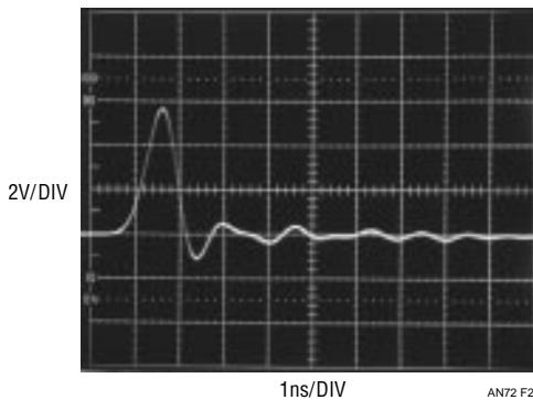
**Figure 27.** Test Pulse on the Same 350MHz Oscilloscope Using a 3GHz 10 $\times$  Probe. Deliberate Poor Grounding Maintains Rippling Residue
