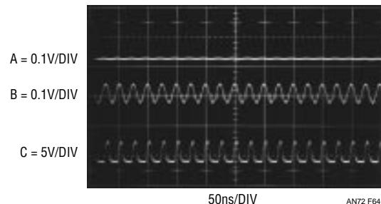
**Figure 64. Adaptive Trigger Responding to a 40MHz, 5mV Input. Input Amplitude Variations from 2mV to 175mV Are Accommodated**
