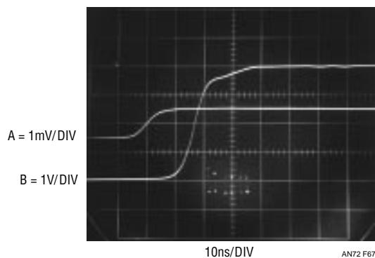
Figure 67. Parallel Path Comparator Shows 18ns Response (Trace B) to  $500\mu\text{V}$  Overdrive (Trace A)
