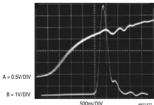
Figure 77. 3.9GHz Sampling Oscilloscope Measures Delay Output and Avalanche Pulse. Pulse-Induced Loading Is Buffered by Ferrite Beads, but Artifacts Appear in Delay Output
