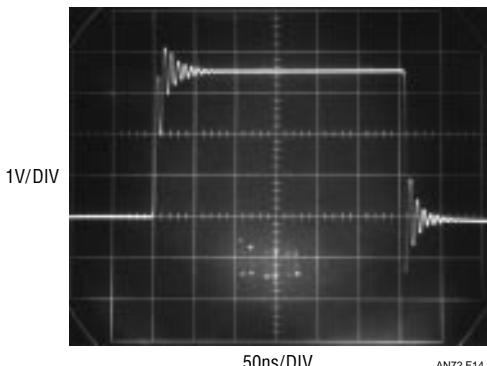
Figure 14. Lengthy, Unterminated Output Lines Ring from Reflections
