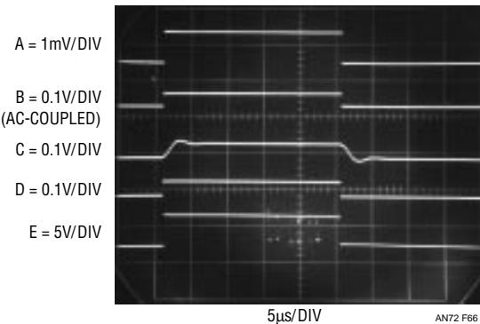
Figure 66.  $500\mu\text{V}$  Input (Trace A) Is Split into Wideband and Low Frequency Gain Paths (Traces B and C) and Recombined (Trace D). Comparator Output Is Trace E
