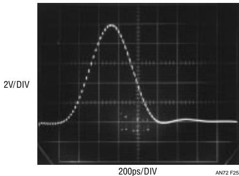
**Figure 25.** A 350ps Rise/Fall Time 10V Pulse Monitored on 1GHz Sampling Oscilloscope. Direct 50 $\Omega$  Input Connection Is Used
