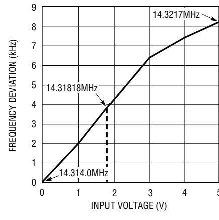
**Figure 52. Control Voltage vs Output Frequency for Figure 51.
