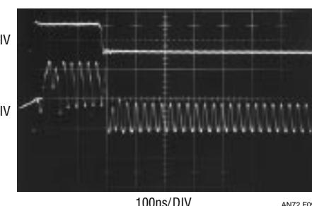
Figure 9. Excessive LT1394 Ground Path Resistance Causes Oscillation
