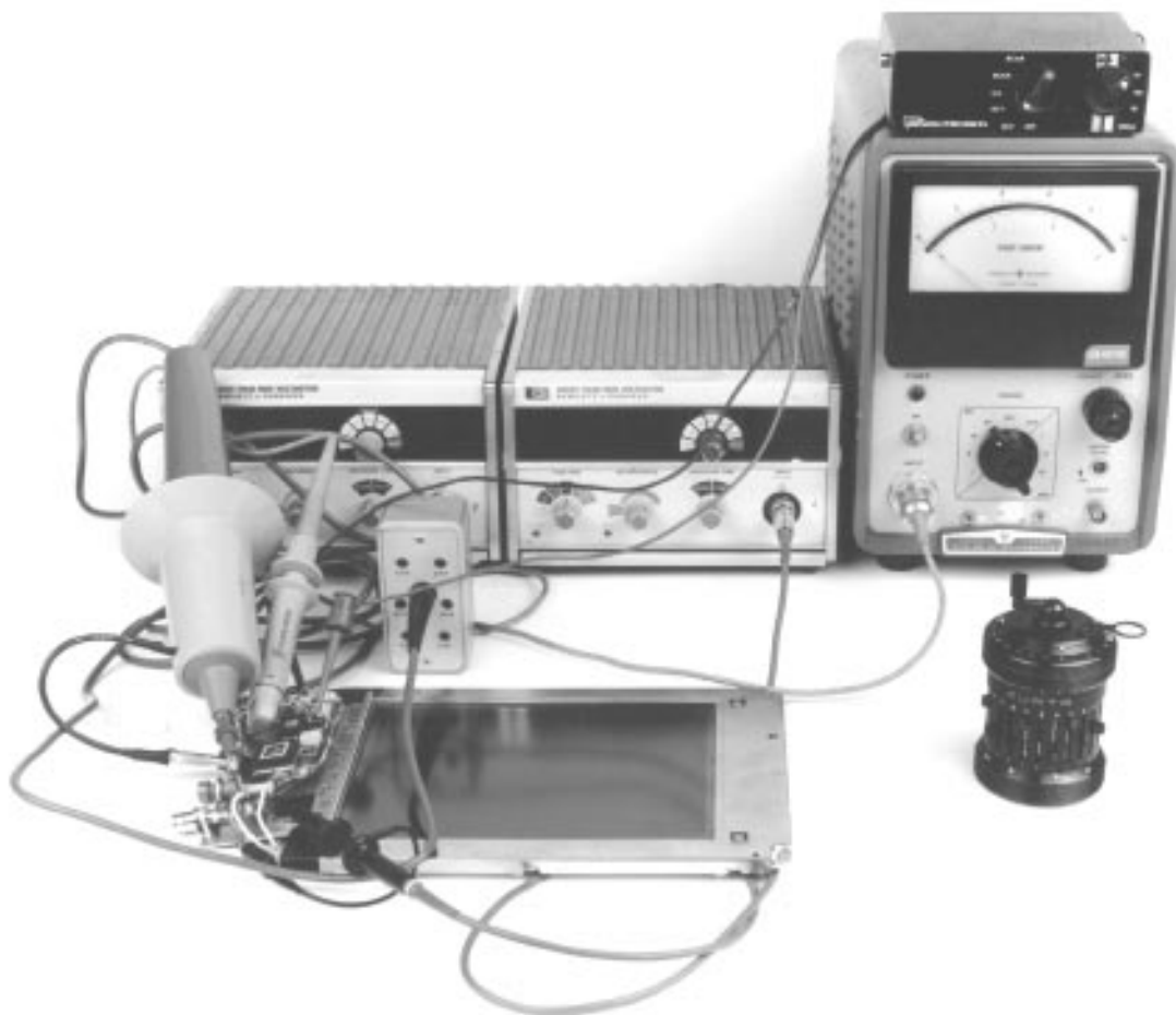
Figure C6. Typical Efficiency Measurement Instrumentation. RMS Voltmeters (Center Left) Measure Output Voltage and Current via Appropriate Probes. Clip-On Ammeter (Right) Gives Low Loss Input Current Readings. DVM (Upper Right) Measures Input Voltage. Hand Calculator (Lower Right) is used to Compute Efficiency
