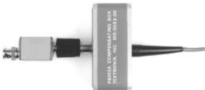
Figure C4. The Impedance Matching Box (Extreme Left) Mated to the High Voltage Probe. Note Direct Connection. No Cable is used
