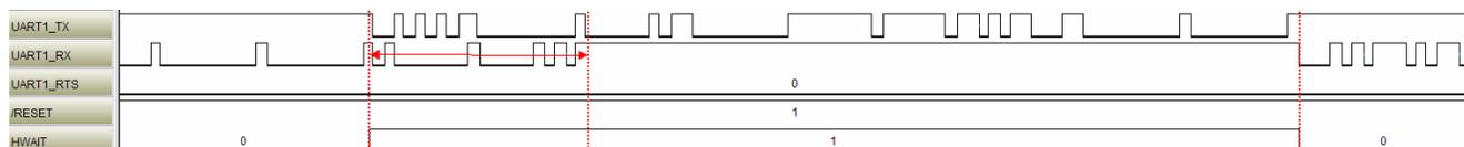
Figure 6. UART: HWAIT signalling
