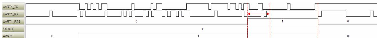
Figure 7. UART: RTS signalling
