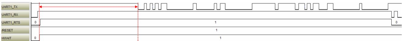
*Figure 9. Manipulation of hardware flow control with additional delay*
