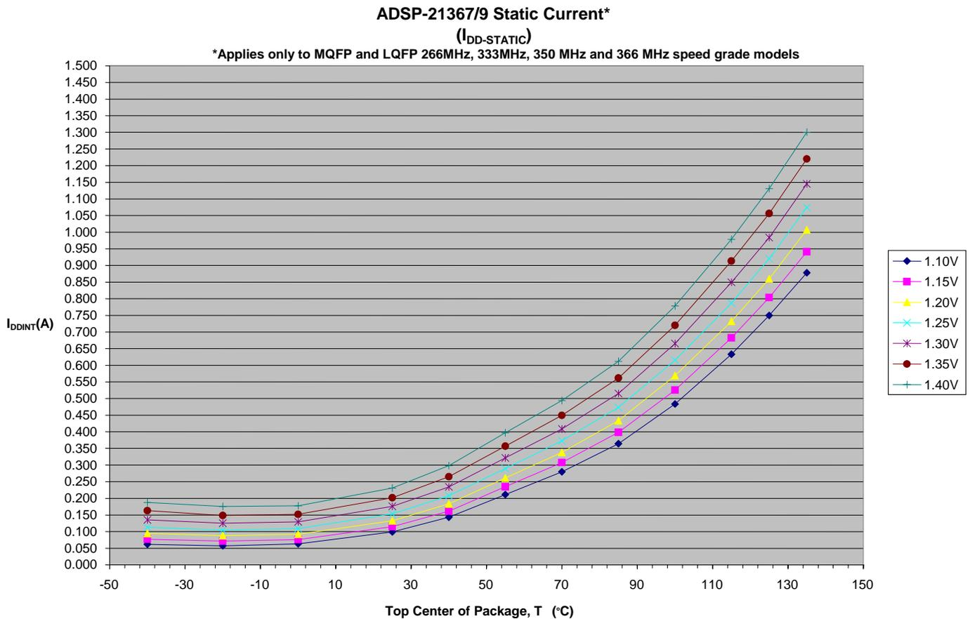
Figure 5.  $I_{DD-STATIC}$  graph
