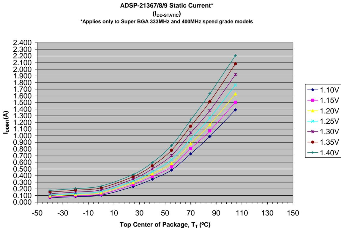
Figure 6  $I_{DD-STATIC}$  graph
