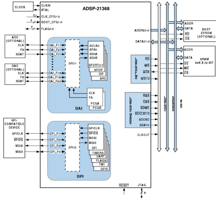
Figure 3. ADSP-21368 system sample configuration
