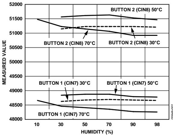
Figure 2. Environmental Effect on Button Sensors
