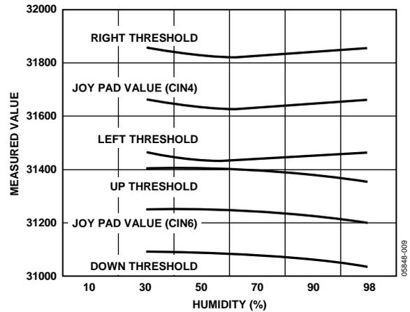
Figure 9. Joy Pad Sensor + Thresholds at Constant 30°C.
