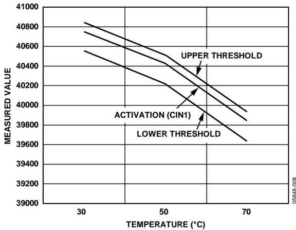
Figure 8. Slider Sensor with Adaptive Thresholds at Constant 50% Humidity
