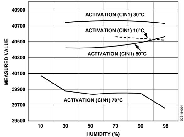
Figure 4. Environmental Effects on Slider Sensor
