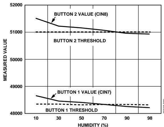
Figure 6. Button Sensors with Fixed Thresholds
