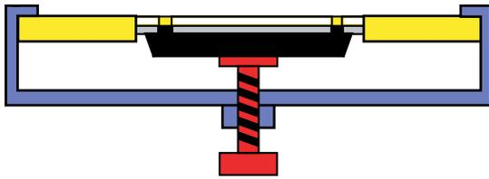
Figure 19. LFCSP is Clamped into Stencil/Jig
