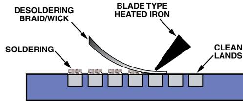
Figure 17. Desoldering the PCB Lands
