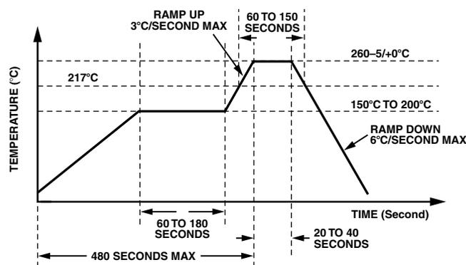
Figure 15. Pb-Free Reflow Profile
