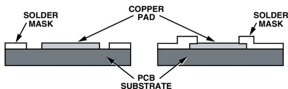
Figure 10. Cross Sections of NSMD and SMD Pads/Land Patterns
