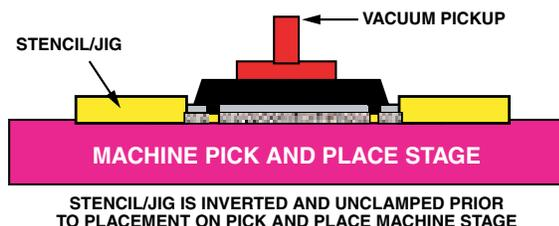
Figure 21. Stencil/Jig is Placed on Rework Machine "Pick and Place" Stage
