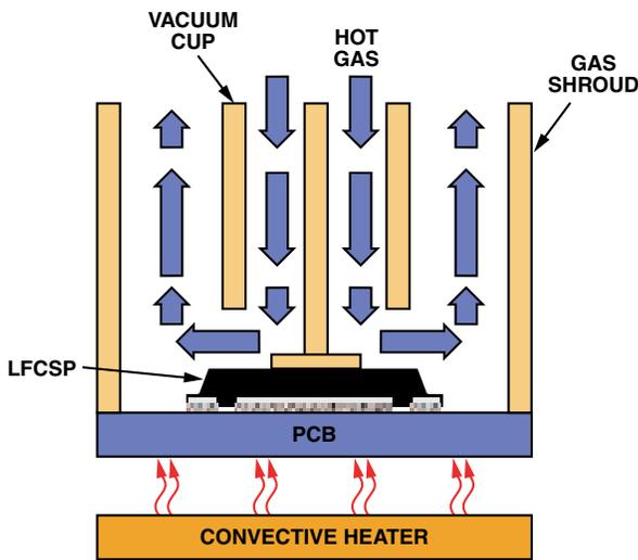
Figure 16. Solder is Reflowed and the LFCSP is Withdrawn Before Solidification
