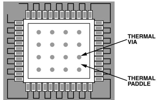
Figure 8. PCB Thermal Paddle and Via
