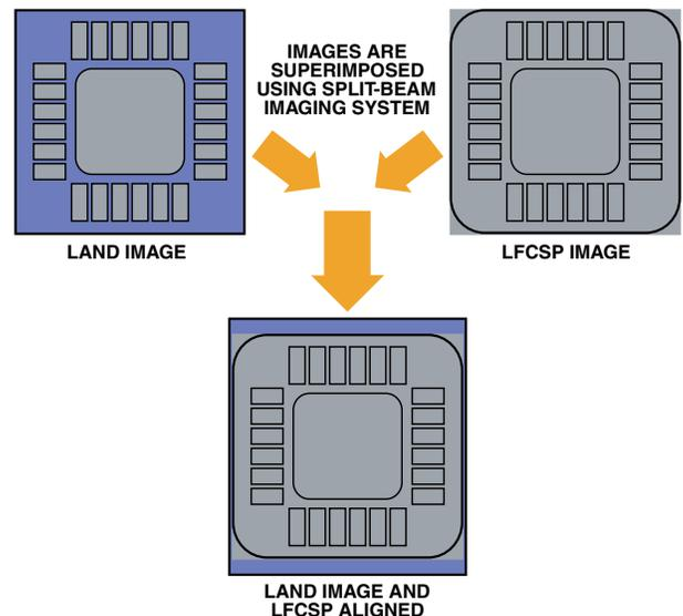
Figure 23. Image of LFCSP is Superimposed onto the Image of the Land Pattern to Facilitate Alignment
