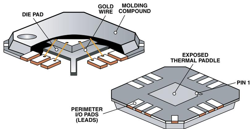
*Figure 1. Isometric Cut Away View of the LFCSP*
