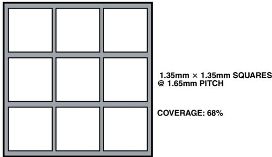
Figure 12. Thermal Paddle Stencil Design for a 7 mm x 7 mm LFCSP Package
