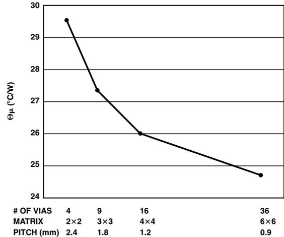
Figure 7. Effect of Number of Thermal Vias on Package Thermal Performance
