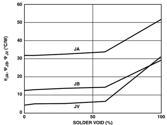
Figure 9. Effect of Voids on Thermal Performance
