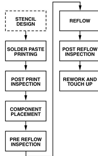
Figure 14. Typical PCB Mounting Process Flow
