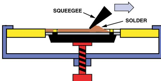
Figure 20. Solder Paste is Applied Through Stencil to the Undersurface of the LFCSP
