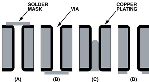
Figure 13. Solder Mask Options for Thermal Vias (a) via tenting from top; (b) via tenting from bottom; (c) via plugging bottom; and (d) via encroach bottom
