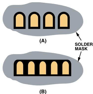
Figure 11. Solder Mask for (A) Perimeter Lands for 0.5 mm and Higher Pitch Parts, and (B) for 0.4 mm Pitch Parts
