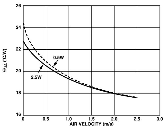
Figure 24. Plots of  $\theta_{JA}$  vs. Air Velocity
