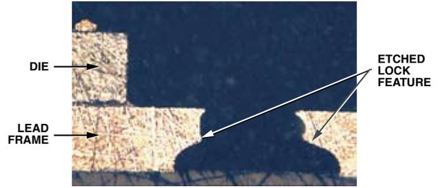
Figure 4. Lead Frame Locking Features
