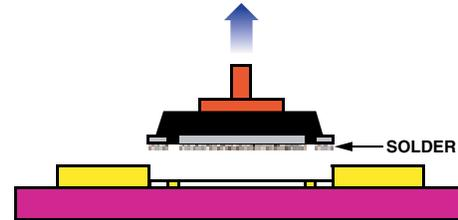
Figure 22. Vacuum Cup Retrieves LFCSP from Stencil Without Disturbing Solder Paste
