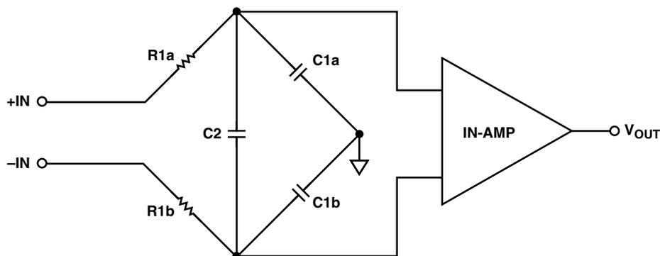
Figure 2. Capacitor C2 Shunts C1a/C1b and Very Effectively Reduces AC CMR Errors Due to Component Mismatching
