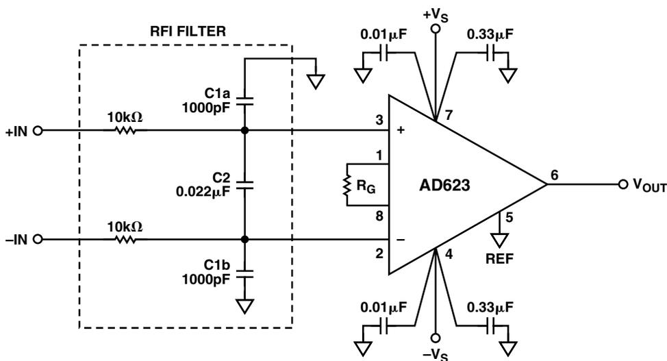
Figure 5. AD623 RFI Suppression Circuit
