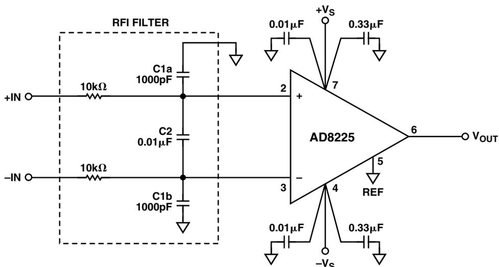
Figure 6. AD8225 RFI Filter Circuit
