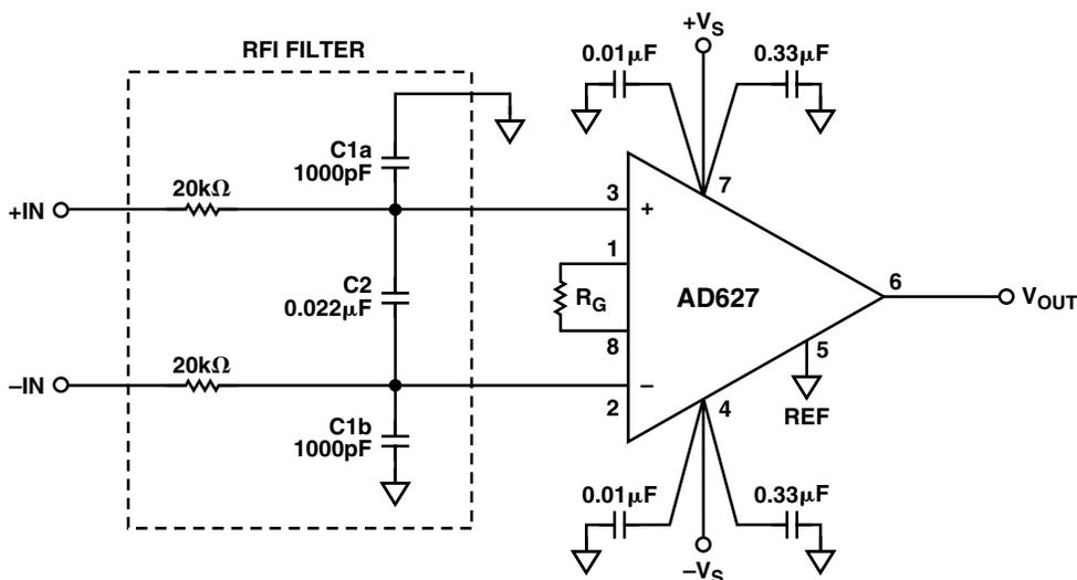
Figure 4. RFI Suppression Circuit for the AD627
