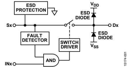
Figure 2. Functional Block Diagram of an OVP Switch
