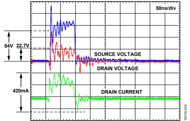
Figure 12. EFT Current for a Single Pulse
