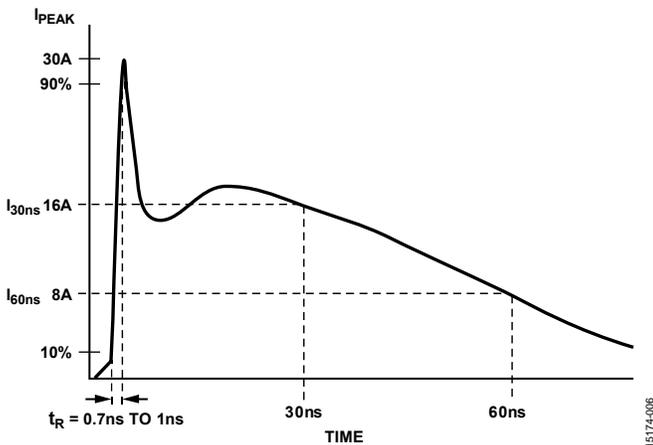
Figure 7. IEC 61000-4-2 ESD Waveform (8 kV)
