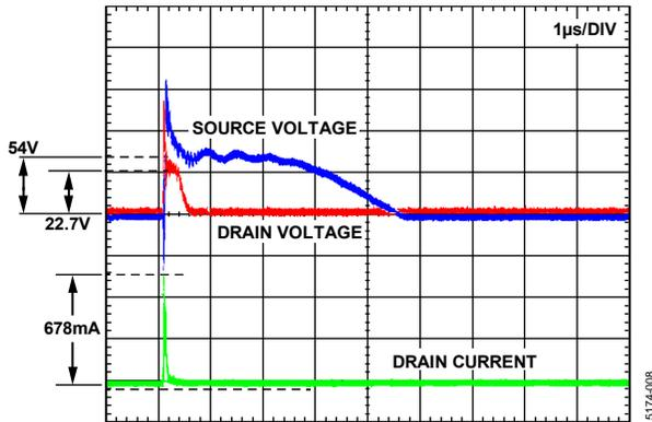
Figure 9. Drain Voltage and Output Current at the Drain (Dx) During an 8 kV Event
