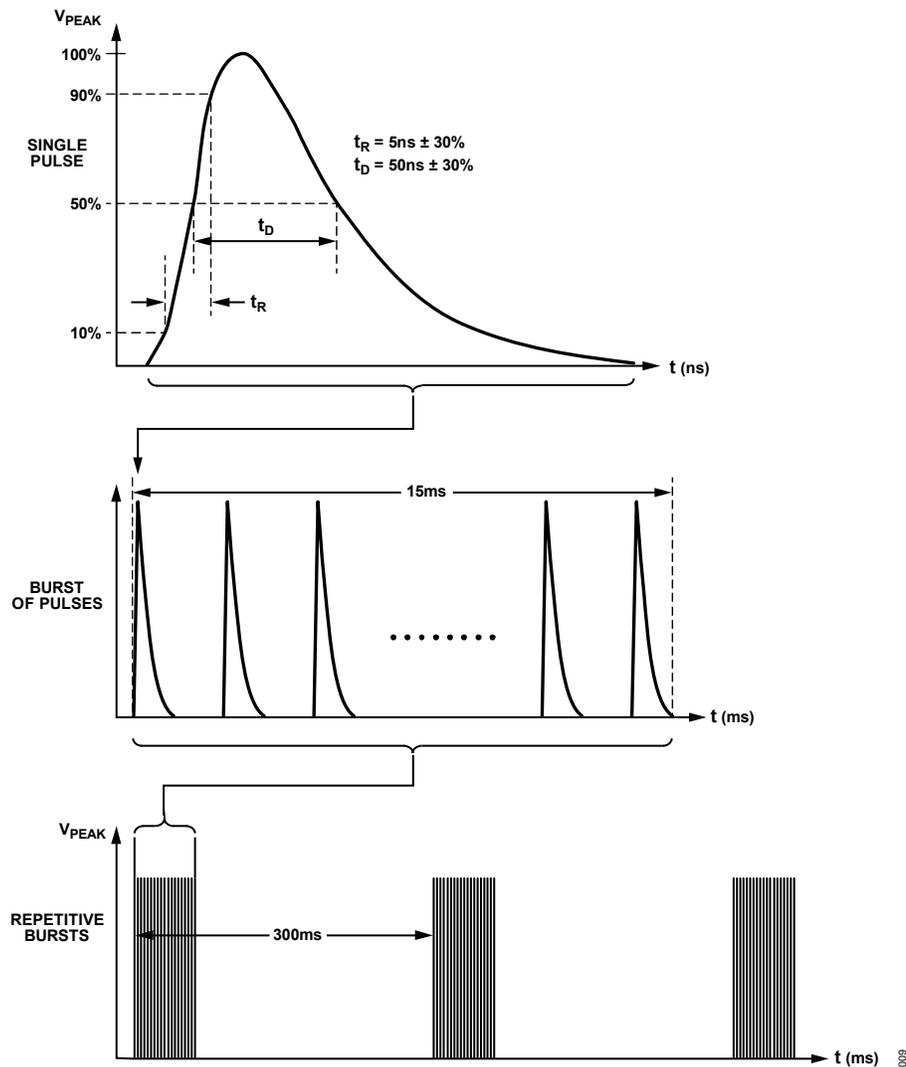
Figure 11. IEC 61000-4-4 EFT Waveform
