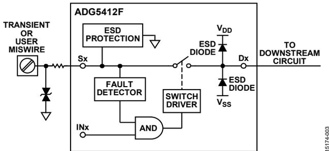
Figure 4. Protection Circuit Diagram
