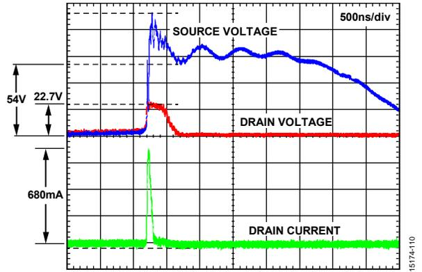
Figure 10. Drain Voltage and Output Current at the Drain (Dx) During a 16 kV Air Discharge Event
