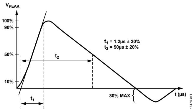
Figure 13. IEC 61000-4-5 Surge 1.2  $\mu\text{s}/50 \mu\text{s}$  Waveform
