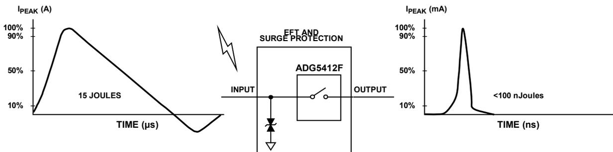
Figure 1. Complete Protection Solution
