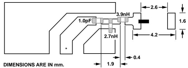
\*LINE WIDTH SHOULD BE DESIGNED TO PROVIDE 50Ω IMPEDANCE MATCHING CHARACTERISTICS.
