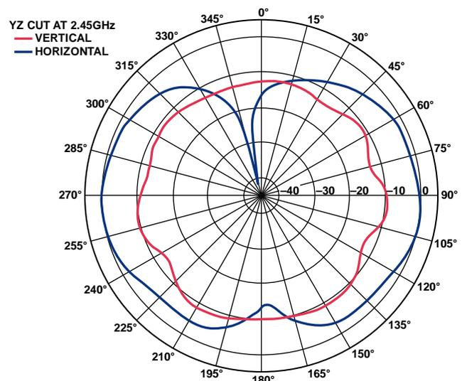
Figure 9. 2450AT18A100 Chip Antenna Typical Radiation Pattern, YZ Cut at 2.4 GHz (25°C)
