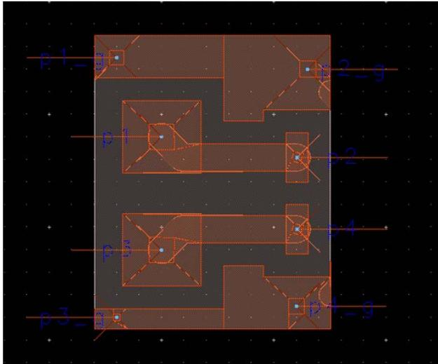
Figure 15. Trace from Decoupling Capacitor to Balun Balanced Port
