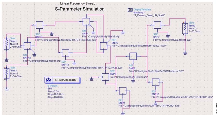
Figure 14. Simulation Equivalent Schematic
