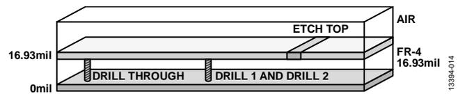
Figure 13. *EVAL-ADF7242-PMDZ* Substrate Material
