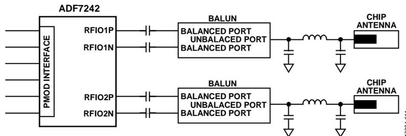
Figure 11. Simplified Connection Circuit Between the [ADF7242](#) and the Chip Antenna
