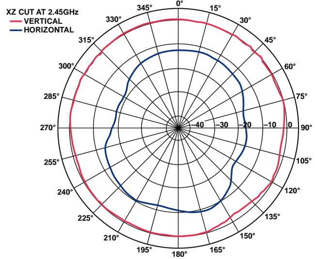
Figure 8. 2450AT18A100 Chip Antenna Typical Radiation Pattern, XZ Cut at 2.4 GHz (25°C)
