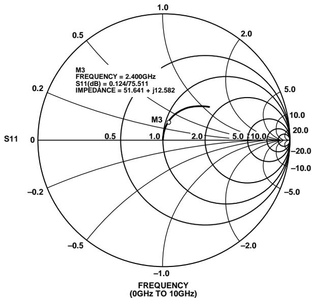
Figure 20. Corresponding Impedance Measurements
