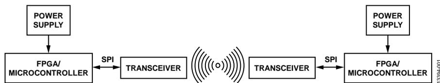
Figure 1. Typical Application Interface System
