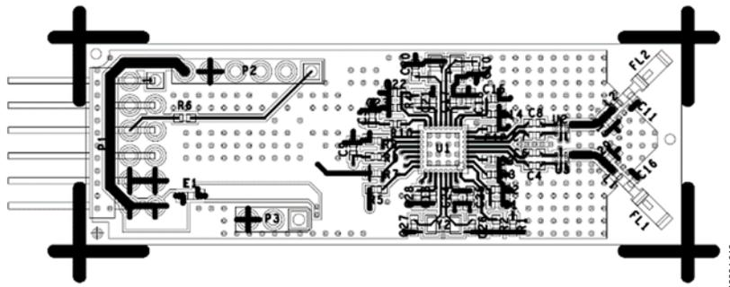
Figure 12. [EVAL-ADF7242-PMDZ](#) Board Layout Highlighting the Chip Antenna Placement
