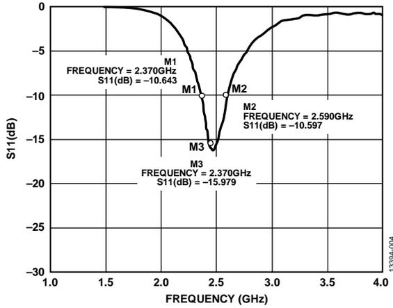
Figure 4. Return Loss with Matching Circuit at 25°C
