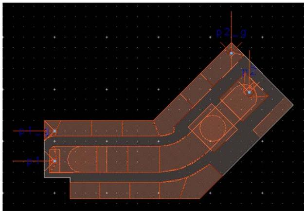
Figure 16. Trace from Balun Unbalanced Port to Matching Circuit
