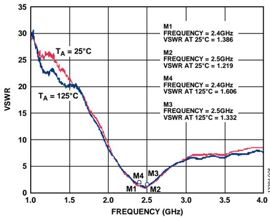
Figure 5. VSWR with Matching Circuit at 25°C and 125°C
