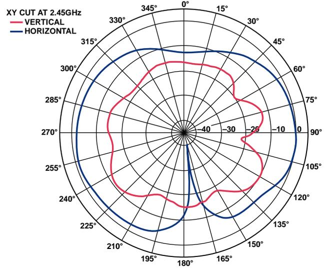
Figure 7. 2450AT18A100 Chip Antenna Typical Radiation Pattern, XY Cut at 2.4 GHz (25°C)
