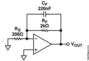
Figure 9. Reducing Noise Using a Feedback Capacitor
