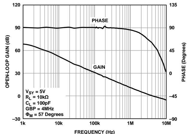
Figure 2. Open-Loop Gain and Phase vs. Frequency
