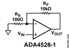
Figure 7. Noninverting Gain Configuration
