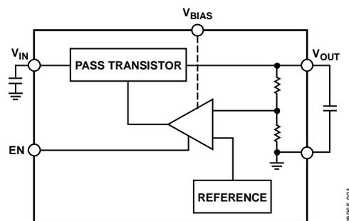
Figure 1. An LDO Regulates the Output Voltage with a Low Dropout Voltage
