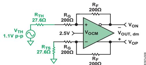
Figure 8. Balanced Single-Ended Termination Circuit
