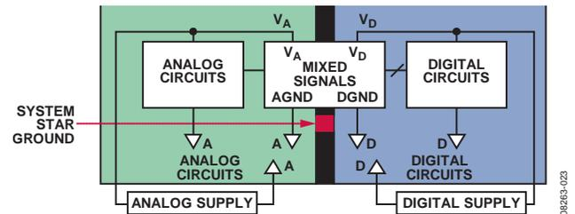
Figure 24. Mixed Signal Grounding
