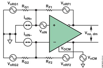
Figure 14. Noise Model of Differential ADC Driver
