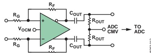
Figure 12. DC-Coupled Inputs with AC-Coupled Outputs
