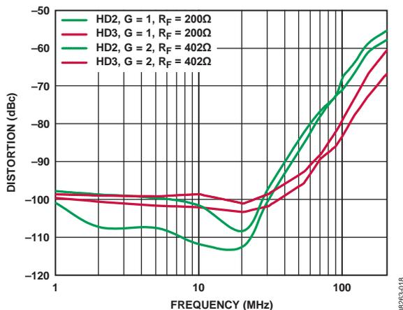
Figure 18. Distortion Curves for ADA4937-1 Current Feedback ADC Driver
