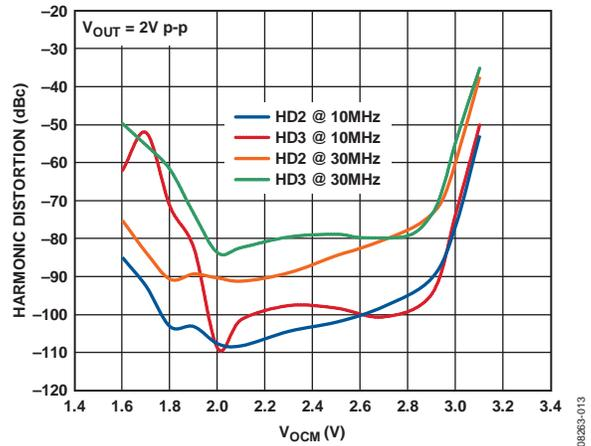
Figure 13. Harmonic Distortion vs.  $V_{OCM}$  at Various Frequencies for the ADA4932-1 with a 5 V Supply
