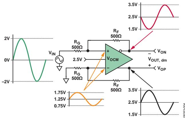
Figure 4. Example of Single-Ended Input to ADC Driver
