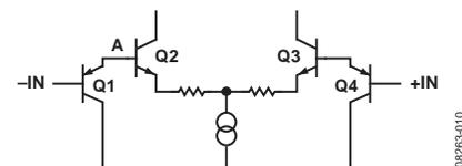
Figure 10. Simplified Differential Amplifier with Shifted ICMVR
