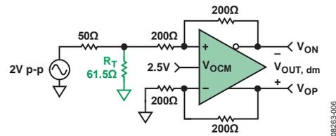
Figure 6. Single-Ended Circuit with Source and Termination Resistances
