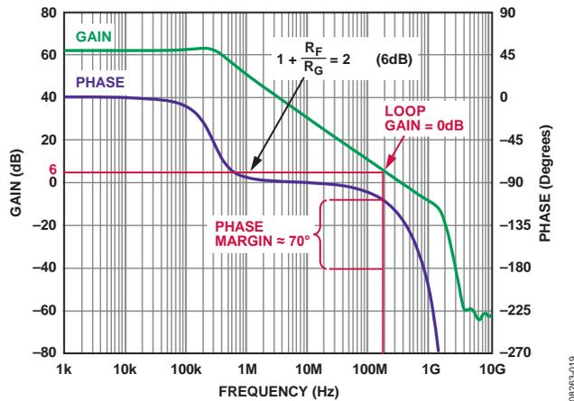
Figure 19. ADA4932-2 Open-Loop Gain Magnitude and Phase vs. Frequency
