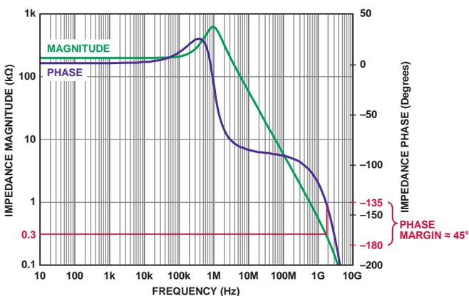
Figure 20. ADA4927-1 Open-Loop Gain Magnitude and Phase vs. Frequency
