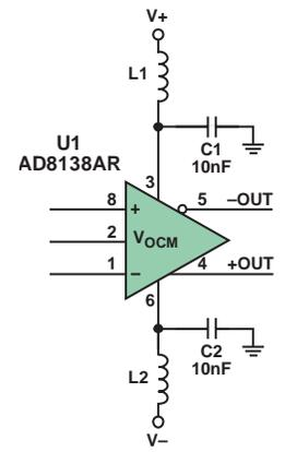
Figure 15. Power Supply Bypassing
