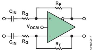
Figure 11. AC-Coupled ADC Driver
