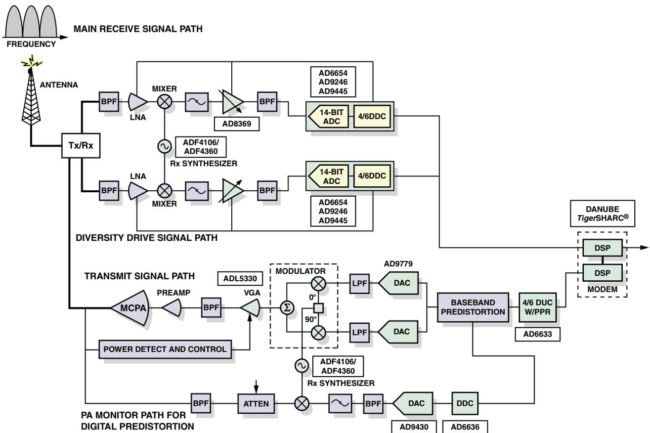
Figure 1. ADI Wideband Multicarrier TRX Common Platform CDMA2000/WCDMA/TD-SCDMA
