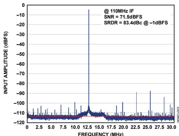
Figure 3. Final Measured Results of the ADC for SNR and SFDR Using the Example Transformer Circuitry
