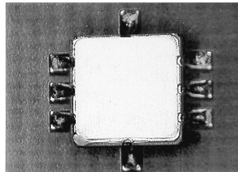
Figure 4. Package-to-Board Alignment (after Reflow)
