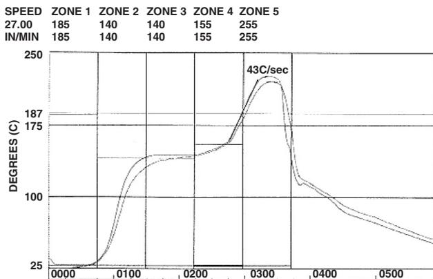
Figure 2. Tests with Standard PbSn Paste Soldering; The LCC Package Supports Standard Reflow Profiles
