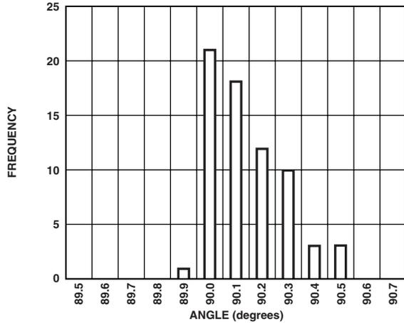
Figure 5. LCC Angle Alignment after Solder; The LCC Package Aligns Very Well to the Pads of the Layout after Reflow Soldering
