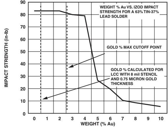
Figure 7. Gold Embrittlement of Solder Joint (Source: "Some Aspects of Soldering Gold Surfaces," C.J. Thwaites, Tin Research Institute, 1973)
