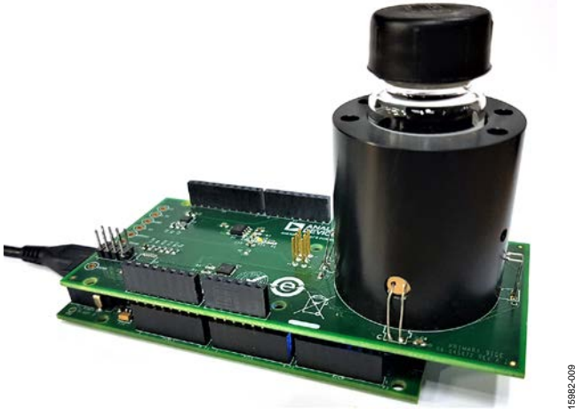
Figure 9. EVAL-CN0409-ARDZ and EVAL-ADICUP360 Water Turbidity Setup
