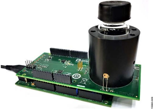
Figure 9. [EVAL-CN0409-ARDZ](#) and [EVAL-ADICUP360](#) Water Turbidity Setup
