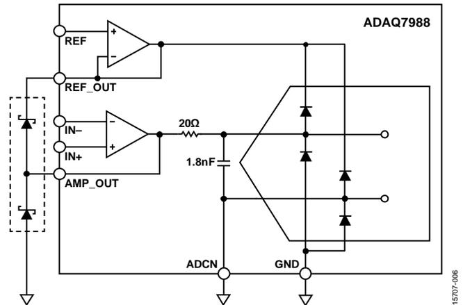
Figure 9. Using Schottky Diodes for Additional Overvoltage Protection
