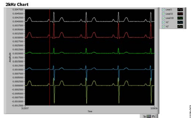
Figure 3. Screen Capture of ADAS1000 with Patient Simulator Connected, Heart Rate = 70 BPM
