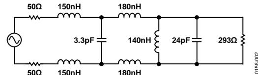
Figure 2. Final Design Values for Fifth-Order Differential Butterworth Filter with  $Z_s = 100 \Omega$ ,  $Z_L = 293 \Omega$ ,  $f_c = 182.5 \text{ MHz}$
