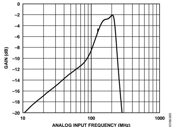
Figure 3. Pass-Band Flatness Performance vs. Analog Input Frequency
