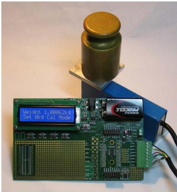
Figure 2. Weigh Scale System Using the AD7191
