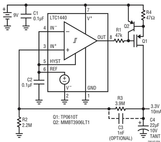
Figure 5. Micropower LDO Regulator
