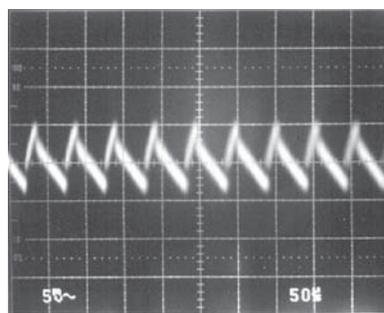
Figure 6. Typical Output Ripple Using 1nF Feedforward Capacitor
