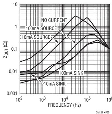
**Figure 5. LT1118-2.5 Output Impedance vs Frequency**
