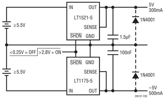
**Figure 2. In a Split Supply Application the Shutdown Pins May Be Comanded in Parallel Using Positive Logic**
