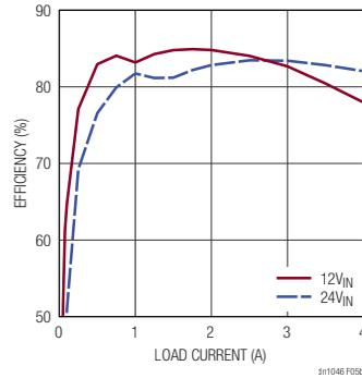
Figure 5. A -5V Supply from a 5V to 35V Input Delivers Current Up to 4A
