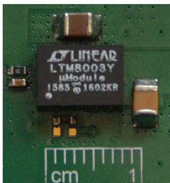
Figure 1. A Complete Step-Down Solution Is Barely Larger than the 6.25mm  $\times$  9mm Footprint of the LTM8003  $\mu$ Module Regulator
