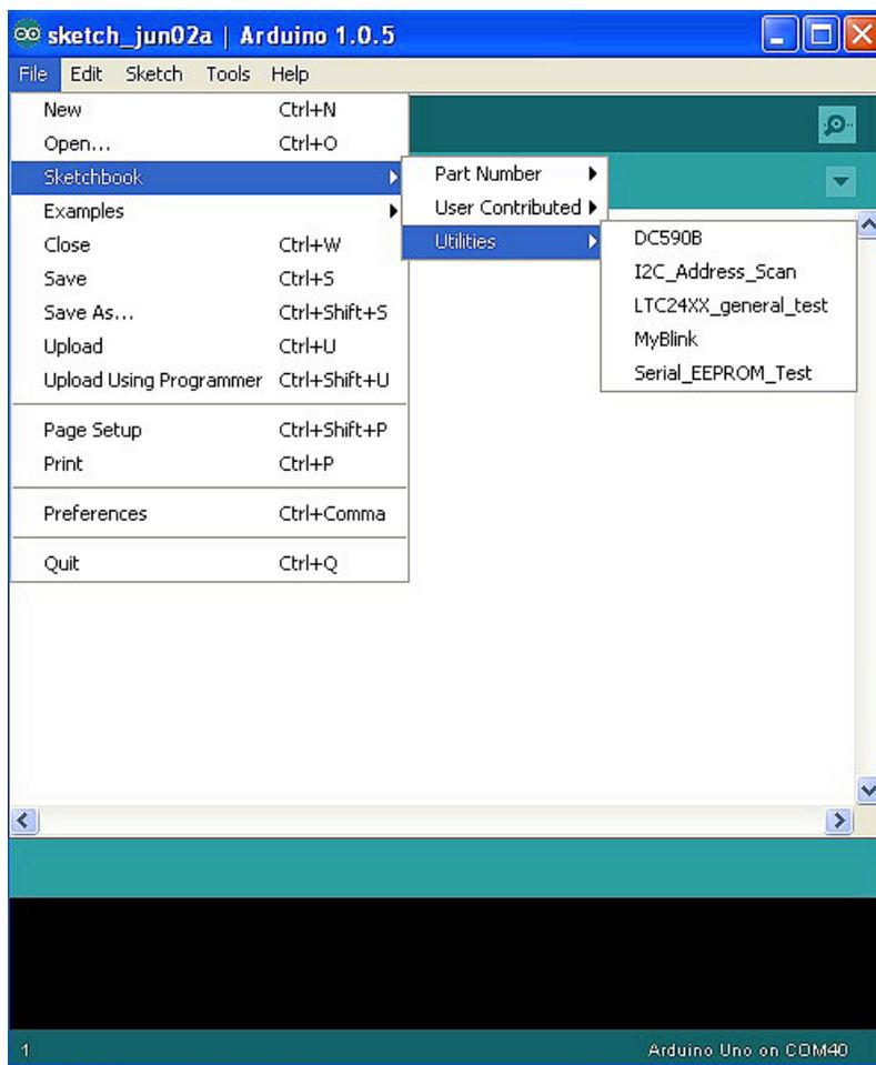
Figure 23. Reloading DC590 Back Into the Linduino
