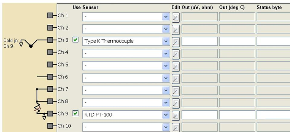
Figure 9. Main Screen After RTD Configuration Was Changed
