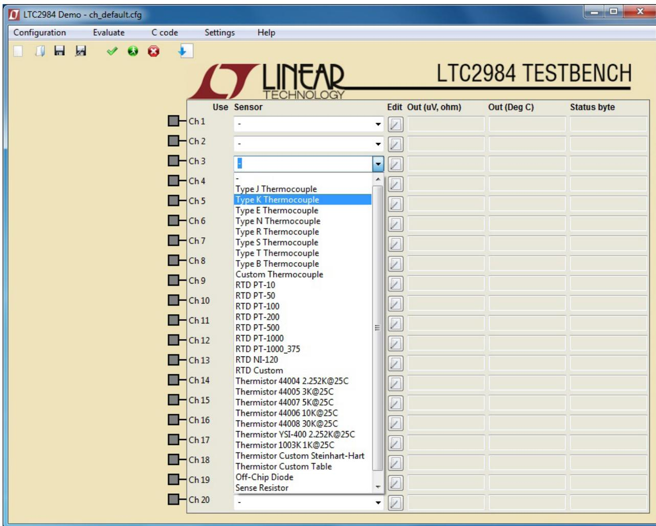
Figure 3. Selecting the Type K Thermocouple
