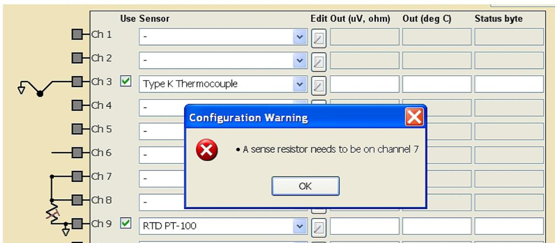
Figure 11. Main Screen After Running the Configuration Checker
