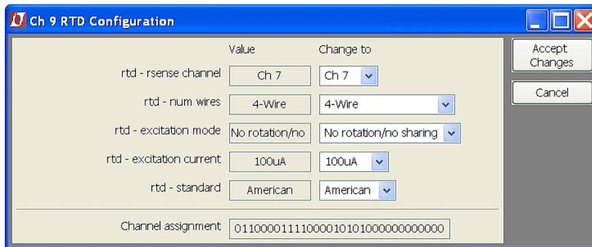
Figure 8. Configuring the RTD on Channel 9
