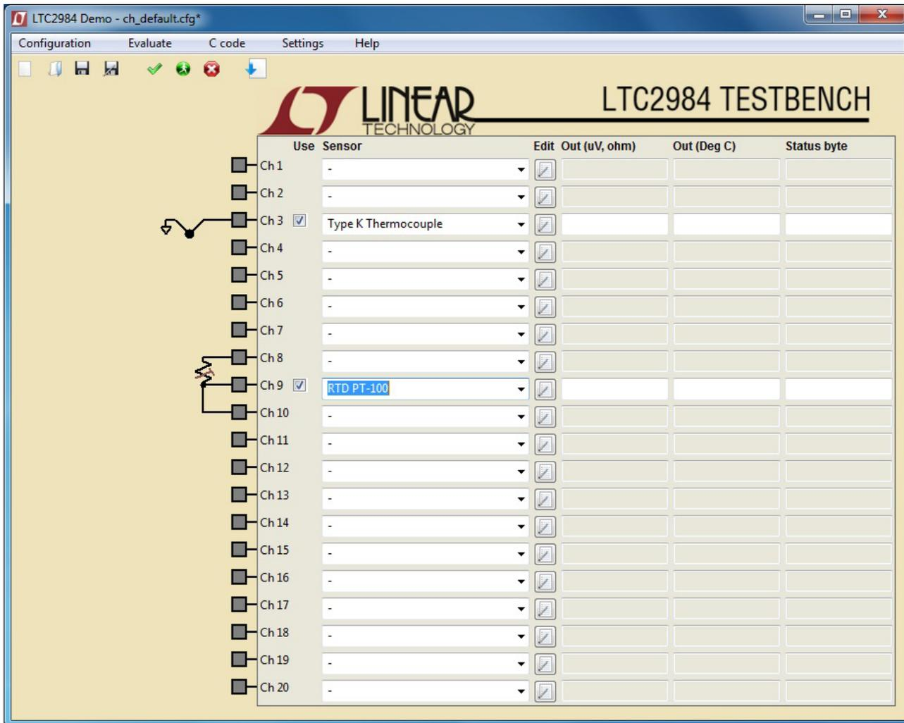
Figure 7. Software After RTD Is Selected on Channel 9
