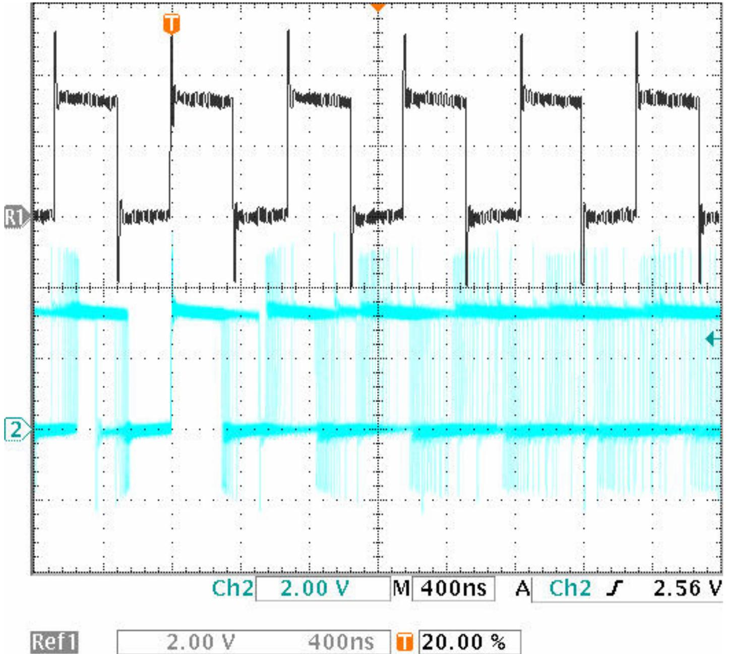
Figure 4. Normal Switching Operation vs. Spread Spectrum Operation
