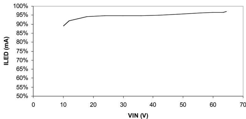
Figure 2. DC1521A Efficiency with 67V LEDs at 370mA
