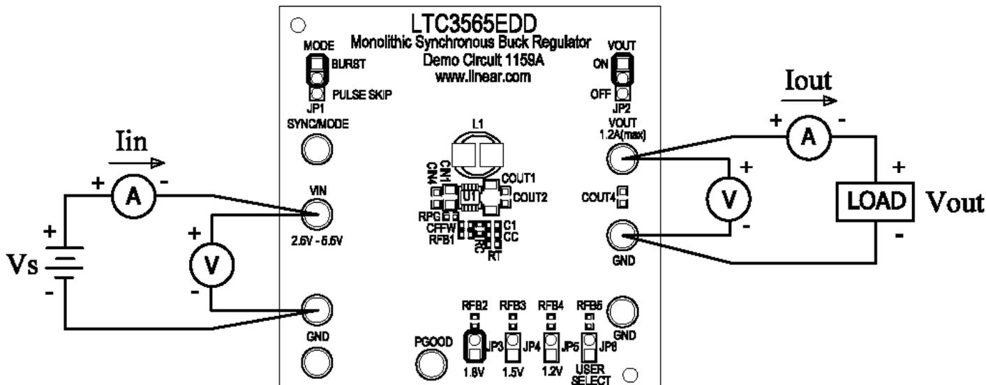
Figure 2. Proper Measurement Equipment Setup
