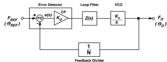
Figure 2. Basic phase-locked-loop model.
