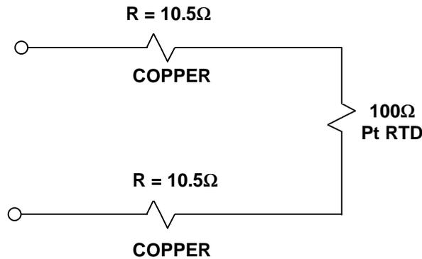
RESISTANCE TC OF COPPER =  $0.40\%/^\circ\text{C}$  @  $20^\circ\text{C}$
