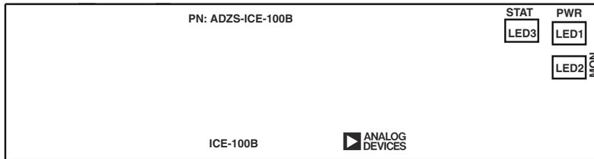
Figure 2-1. LED Positions - Top of Emulator Board
