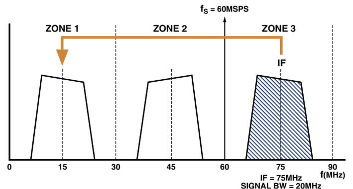
Figure 18. Sampling a 20-MHz BW signal with an IF frequency of 75 MHz at a sampling rate of 60 MSPS.
