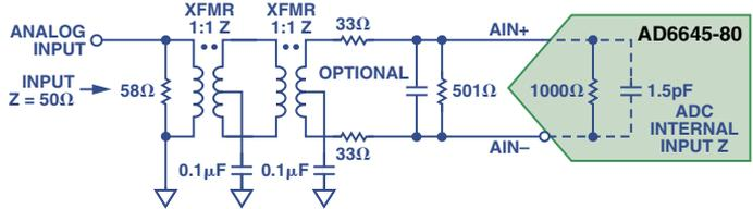
Figure 4. Cascaded transformers.
