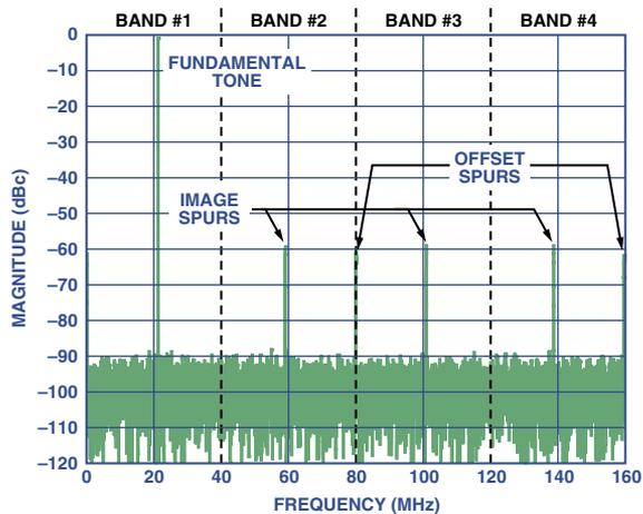
Figure 5. 4-channel time-interleaving FFT.
