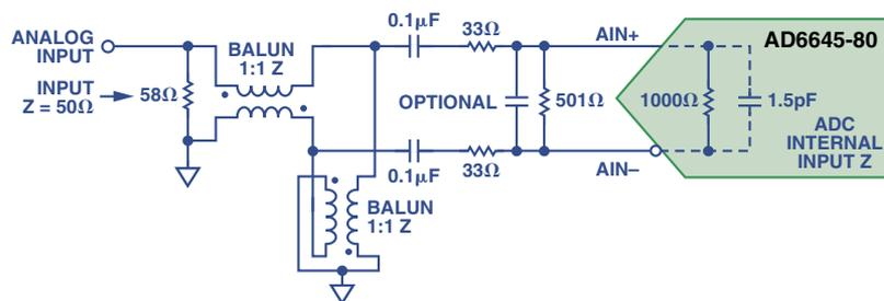
Figure 7a. Transformer-coupled input using a two-balun type transformer configuration.
