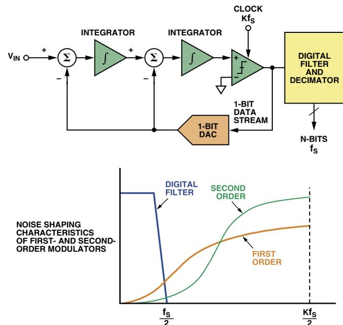
Figure 8. Second-order  $\Sigma$ - $\Delta$  modulator.
