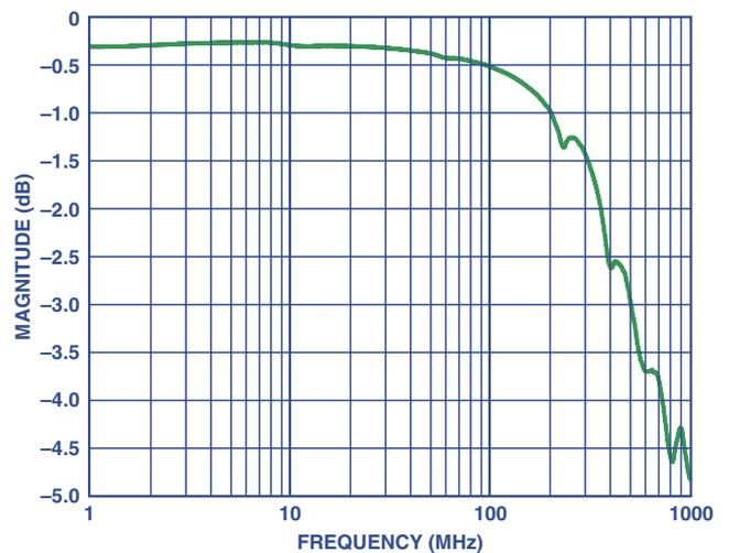
Figure 8a. Frequency response of a typical transformer.
