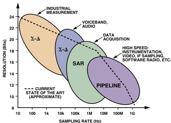
Figure 1. ADC architectures, applications, resolution, and sampling rates.
